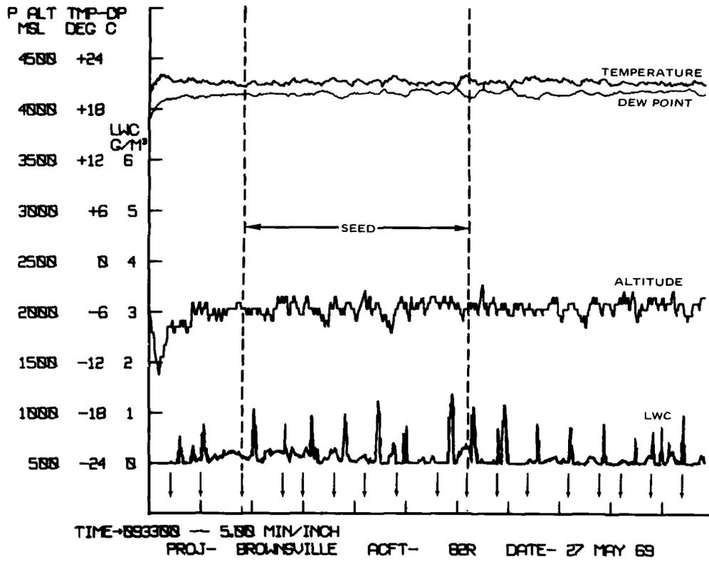
FIG. 11. Computer Plot of Liquid Water Content, Temperature, Dew Point, and Altitude Versus Time. Test 14, 27 May 1969. Arrows denote times of initial cloud penetration. Liquid water content as portrayed is three times greater than actual because of computer programming requirements.
